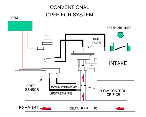
The Delta Pressure Feedback EGR Monitor is a series of electrical tests and functional tests that monitor various aspects of EGR system operation.
